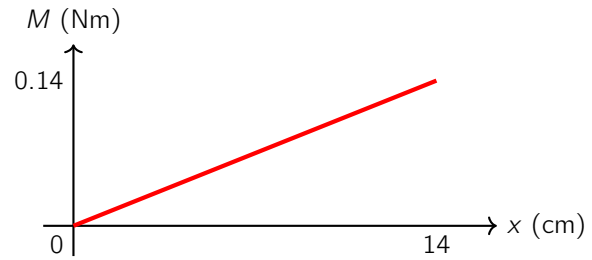
(b) Bending Moment Diagram M(x)
